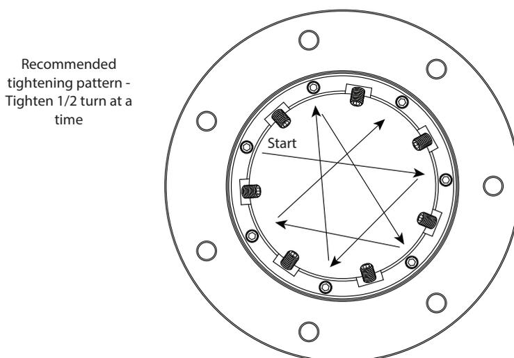
**NOTE: Keep tightening until ALL the bolts are at the required torque setting. Bolts that have reached the required torque can loosen when other bolts are tightened.**
