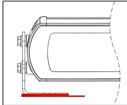
2. Before permanently installing the light, find a suitable position that preferably avoids "Bow Glare". Using a piece of string from the bow of the boat to the top of the light (or draw an imaginary line) (fig 3), place and adjust the tilt of the light so that no light falls on to the bow (fig 4 & 5).
