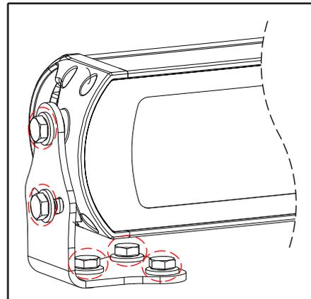
8. Return the light to the marked angle (fig. 18). Bolts on the sides of each bracket can now be tightened to a final torque of 8Nm. Only once the light has been angled and side bolts tightened can the brackets be tightened down.
