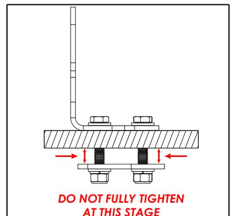
7. Mount light to brackets using the fixing hardware from step 1 (note the location of the nylon washer). It is recommended to fit the top bolt on both sides first before fitting the angle lock bolt. Note: All bolts at this point should still be loose.
