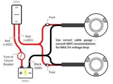
The light cables can be extended. Ensure the correct cable gauge is used to avoid issues with voltage drop. Follow ABYC recommendations for no more than 3% voltage drop. Consult a qualifed electrical installer, or contact Lumishore for further information.
