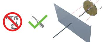
IMPORTANT: Do Not Over Tighten. **Do Not Use Power Tools to tight**en screws.
