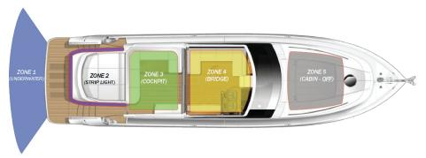
Create the five separate lighting zones and select the desired color and intensity for each one.
