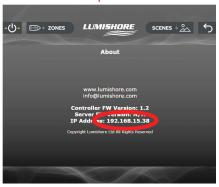
Type the IP address into the browser on the smart device or laptop.
