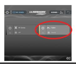
Press the power icon to turn each zone on/off press the right hand side of tab to enter main control page.
