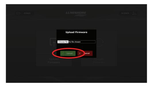
Once the file has uploaded you can choose to install now or install at a later time. Select install now to complete the firmware update. (the process can take 30-50 minutes), please ensure the PC or laptop and Lumi-Link Command Center are left uninterrupted during this time.
