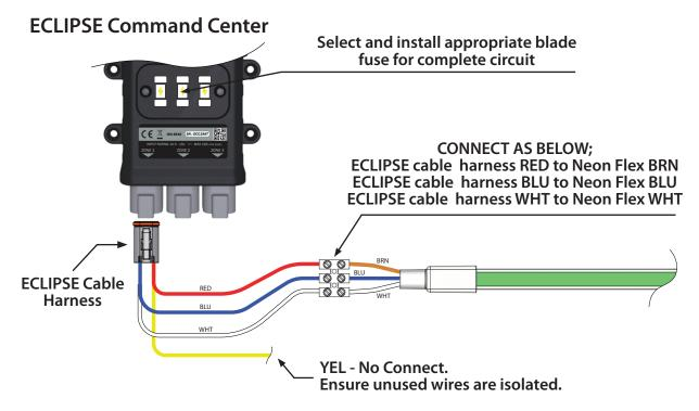
Note: Single color and dual color lights should not be added to the same zone output. Use a separate zone output for each type.
