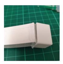
8. Fit end cap over extrusion and push until it stops. Excess adhesive should be wiped away using water ONLY. Use a paper towel to dry and allow to cure undisturbed for 24hrs.
