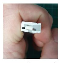
6. Cut a 4mm piece of sponge cord (included) and place inside cavity. Push the cord down until it is flush with the end of the extrusion. The sponge cord prevents the sealant from touching the LED's which may cause color shift.
