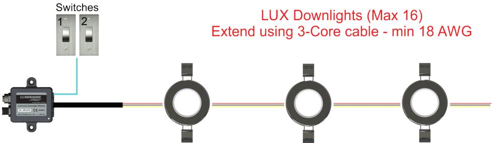
**NOTE: The Lumishore Lux downlight DL50 requires connection to the Lumishore Lux Downlight Module. For full electrical installation and wiring diagrams please refer to the Lux Downlight Module installation guide.**
